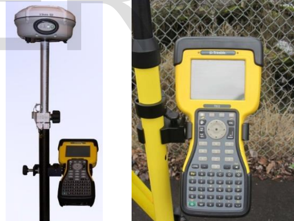
Fig. 3: GNSS Trimble R8 receiver (left) and Trimble TSC2 Controller (right) [3]
